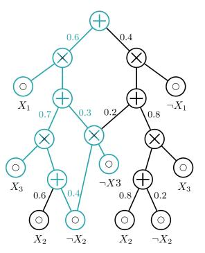
Any parts of circuit not relevant for MMAP state can be pruned away
