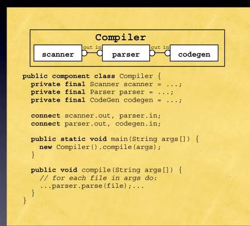
connect: this primitive connects two or more ports together, binding each required method to a provided method with the same name and signature.
