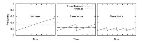
Figure 3. A graphical representation of routing-table reset, with increasing frequency from left to right graphs.
