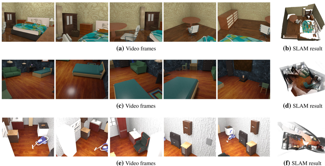
Fig. 10 Specifying camera trajectories, we can render scene fly-throughs as sequences of video frames, which may be used to evaluate SLAM reconstruction (Whelan et al. 2015) results; e.g., a, b a successful reconstruction case and two failure cases due to c, d a fast moving camera and e, f untextured surfaces
