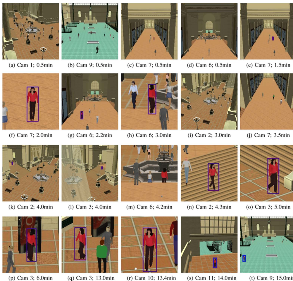
Fig. 18. 15-min persistent observation of a pedestrian of interest as she makes her way through the train station (refer to Fig. 17). (a)–(d) Cameras 1, 9, 7, and 8 monitoring the station. (e) The operator selects a pedestrian of interest in the video feed from Camera 7. (f) Camera 7 has zoomed in on the pedestrian. (g) Camera 6, which is recruited by Camera 7, acquires the pedestrian. (h) Camera 6 zooms in on the pedestrian. (i) Camera 2. (j) Camera 7 reverts to its default mode after losing track of the pedestrian and is now ready for another task. (k) Camera 2, which is recruited by Camera 6, acquires the pedestrian. (l) Camera 3 is recruited by Camera 6; Camera 3 has acquired the pedestrian. (m) Camera 6 has lost track of the pedestrian. (n) Camera 2 observing the pedestrian. (o) Camera 3 zooming in on the pedestrian. (p) Pedestrian is at the vending machine. (q) Pedestrian is walking towards the concourse. (r) Camera 10 is recruited by Camera 3; Camera 10 is observing the pedestrian. (s) Camera 11 is recruited by Camera 10. (t) Camera 9 is recruited by Camera 10.
