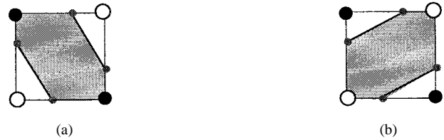
Fig. 4. (a) and (b) Example of ambiguous faces of a cube (black circle: positive cell vertex, open circle: negative cell vertex). Given the diagonal arrangement of vertex polarities, it is unclear which edge/surface intersection should be used.
