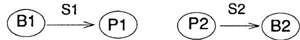
Figure 7: A two cell configuration where both pads are in range of their respective base stations and also in range of each other. Base station B1 is sending data to pad P1, and pad P2 is sending data to base station B2. Each stream is generating data at a rate of 64 packets per second and using UDP for transport.
