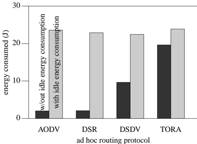
**Figure 1: Comparison of energy consumed for four ad hoc routing protocols with different energy models (left, black bars are without considering energy consumed when listening; right, gray bars include this consumption). The simulation has 50 nodes in a 1500m\*300m area. Nodes move according to the random way-point model. The energy model is based on Stemm and Katz [30].**
