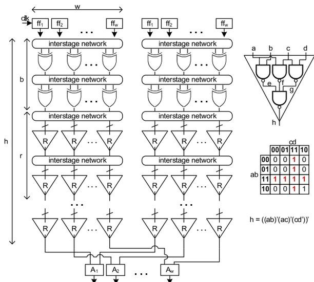
Figure 2: dPPUF architecture of height  $h$  and width  $w$ . A challenge vector propagates through repeated layers of  $b$  booster (XOR) and  $r$  repressor (R) cells (right), with partly maximally interacting and partly random interstage networks. Signals from 2 nominally identical but physically unique PUFs race to arbiters ( $A_i$ ) to produce the response.
