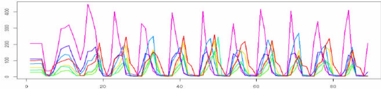
**Figure 1 :** Data from 7 pressure sensors embedded in the Smart Shoe. The system performs signal processing, feature extraction on streamed pressure data, and incorporates results from both shoes to assess fall risk.
