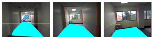
**Figure 5.** Consecutive image frames showing the decreasing height of the detected floor region as the user approaches the end of the corridor.
