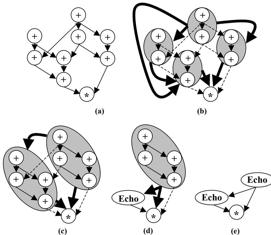
**Fig. 5.** A DFG (a) with a set of patterns replaced by supernodes (b), after a second iteration (c), and with one of the supernodes replaced with an echo instruction (d). If the pattern existed elsewhere in the program, both could be replaced with echo instructions (e)
