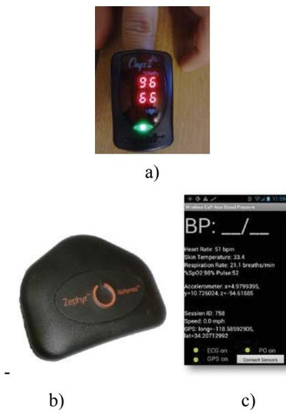
Figure 3. Virtual Cuff Sensor and Interface. a) Nonin Onyx II 9560 Fingertip Pulse Oximeter used on the finger to derive PPG signals. b) Zephyr Bioharness strapped to the users chest collects ECG data. c) Screen Shot of Android App
