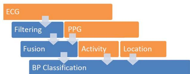
Figure 2. Virtual Cuff Sensor and Component Interaction Overview
