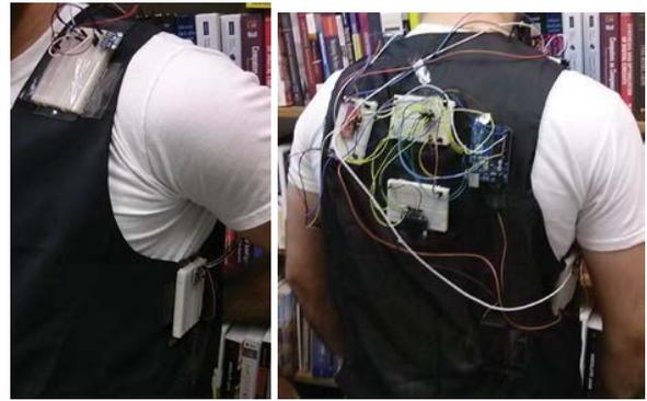
**Figure 4. Image of LightVest, including Arduino Uno microprocessor and four light panels from front and back.**
