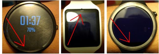
**Figure 2. Identification of smart watch ambient light sensor location, for three commercially available smart watches (Moto360 1st Generation, Sony 3, and Moto360 Sport, from left to right).**
