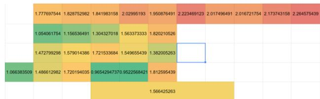
**Figure 9.** Heat map of the average lux readings for the numbers, letters, space bar, and left shift key. Colors reflect lux value, with red being larger and green being smaller.
