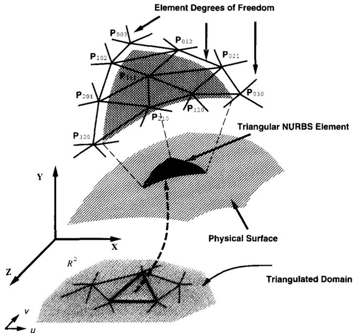
Fig. 2. One finite element and its degrees of freedom of a triangular NURBS surface.
