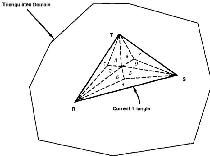
Fig. 3. Nine subtriangles for numerical quadrature.
