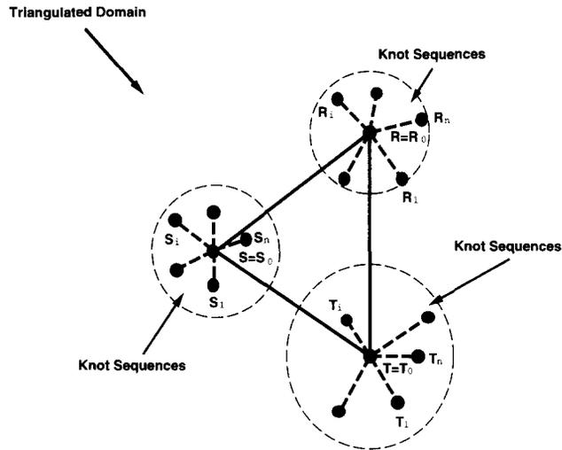
Fig. 1. Knot vectors associated with each triangle in the domain triangulation.
