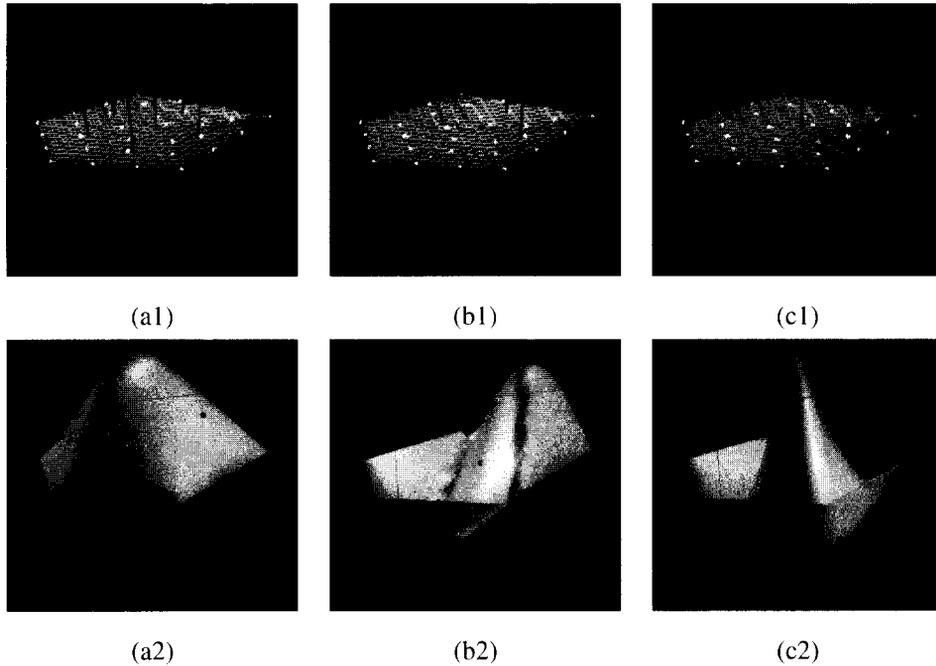
Fig. 10. Fitting a pentagonal surface to three different sets of scattered data. Data points and initial surfaces (a1,b1,c1). Final fitted surfaces (a2,b2,c2).
