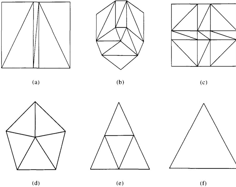
Fig. 6. Domain triangulation of surfaces used in the examples (see text). (a) An edge. (b) A trihedral corner. (c) A bevel joint. (d) A pentagonal surface. (e) An open quadratic surface. (f) A cubic patch.
