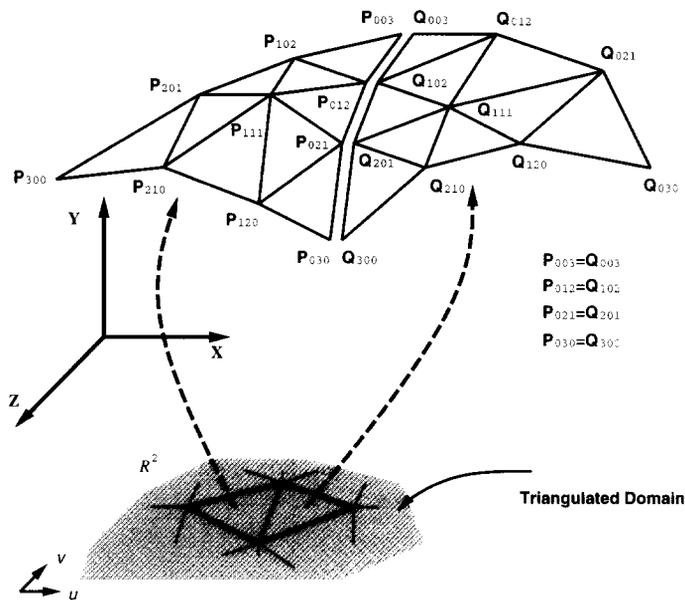
Fig. 5. A constrained triangular B-spline configuration: *continuous net*.
