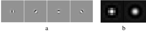
Figure 4: (a) Four basis filters oriented at 0^\circ , 45^\circ , 90^\circ , and 135^\circ . (b) Left: L_1 low-pass filter, Right: L_0 low-pass filter.
