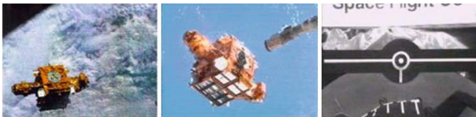
Fig. 1 Images acquired during satellite capture. The left and center images were captured using the shuttle bay cameras. The right image was captured by the end-effector camera. The center image shows the shuttle's manipulator arm in hovering position prior to the final capture phase. The shuttle
