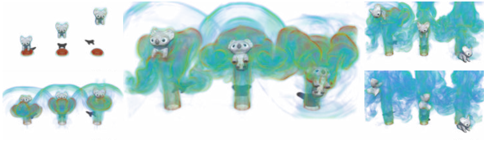
Figure 3.19: Demo: Three koala toys hit by Mach diamond jets. The inlet setting mimics the 2D version in Figure 3.18. The density ratio (from left to right) of the koalas is 1:4:9. The lightest koala is easily propelled upward; the middle one maintains balance under the effects of the pumping jet and gravity; the heaviest koala easily disrupts the jet's wavefront.
