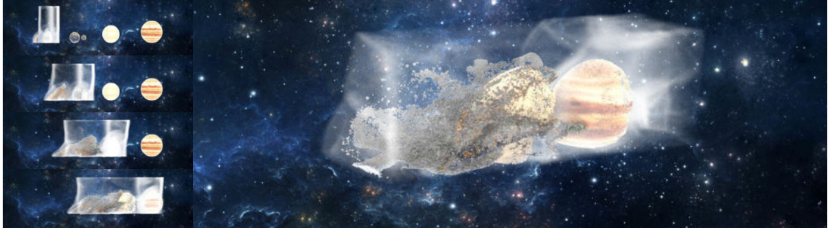
Figure 3.14: Demo: Supernova. A supernova destroys multiple planets, producing a massive amount of fragments in a mini solar system. This example contains numerous complex solid-fluid interfaces with a wide range of solid volume fractions. Our partially passable interface treatment robustly handles them.
