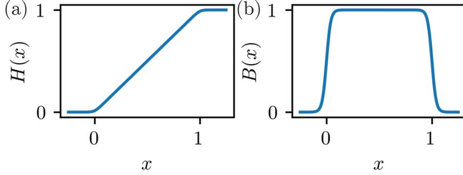
Figure 3.2: (a) Smooth approximated fixbound function  $H(x)$ , which models the piecewise function in (3.12). (b) Boxcar function  $B(x)$ , which allows for an analytical conditional reassignment. Both functions are plotted with a stiffness parameter of  $k = 50$ .
