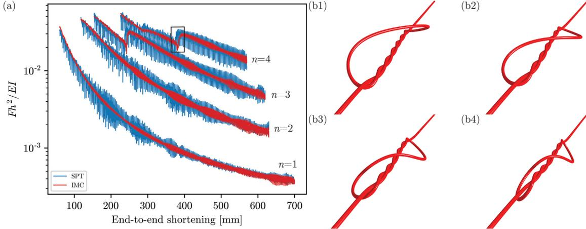
Figure 4.2: Simulation results comparison. (a) Pull force comparison for unknotting numbers 1 through 4 using SPT (Spillmann and Teschner, 2008) and IMC with  $u = 6$  mm/s,  $\Delta t = 0.5$  ms, and  $\mu_k = 0.10$ . (b) Inversion occurring for  $n = 4$  and the corresponding drop in pull forces shown by the border box in (a).
