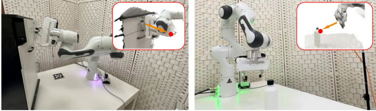
Figure 4.4: Real-world experiments with inference results shown on the upper right. The red dots indicate the predicted positions of the next action for the end-effector.
