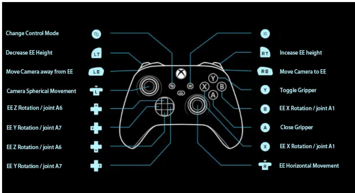
Figure A.10: A schematic of the Xbox controller
