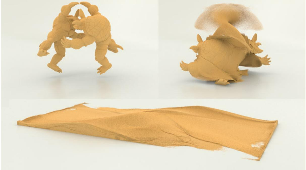
Figure 3.11: **Sand armadillo.** In this simulation, two sand armadillos hug and smash together using 4 GPUs with 55M particles and a grid resolution of  $512 \times 512 \times 1024$ . Fine details are captured with a small  $\Delta x$ .
