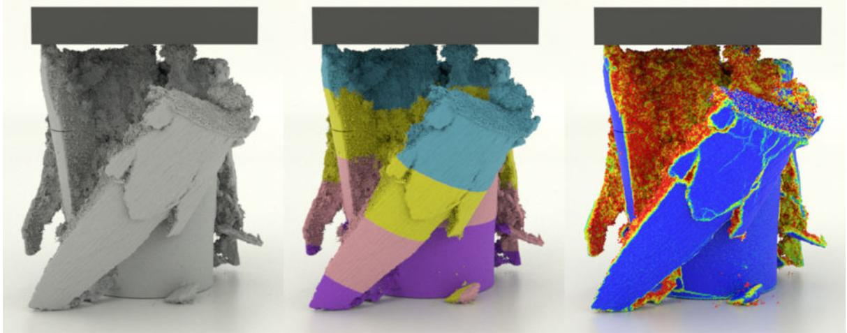
Figure 3.1: **Crushing concrete.** Our system enables this concrete crushing simulation (inspired by the hydraulic press) on a single workstation with 4 NVIDIA Quadro P6000 GPUs. This simulation contains 93.8 million particles on a  $1024^3$  grid, achieving a 3.9 min/frame performance. (Left) A concrete-style render. (Middle) Coloring by GPU. (Right) Coloring by the plastic volumetric strain for visualizing the damage propagation.
