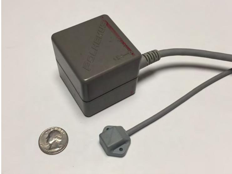
Figure 4.12: Our Polhemus magnetic tracker. A smaller, cheaper alternative to the Ascension tracker (Figure 4.2).
