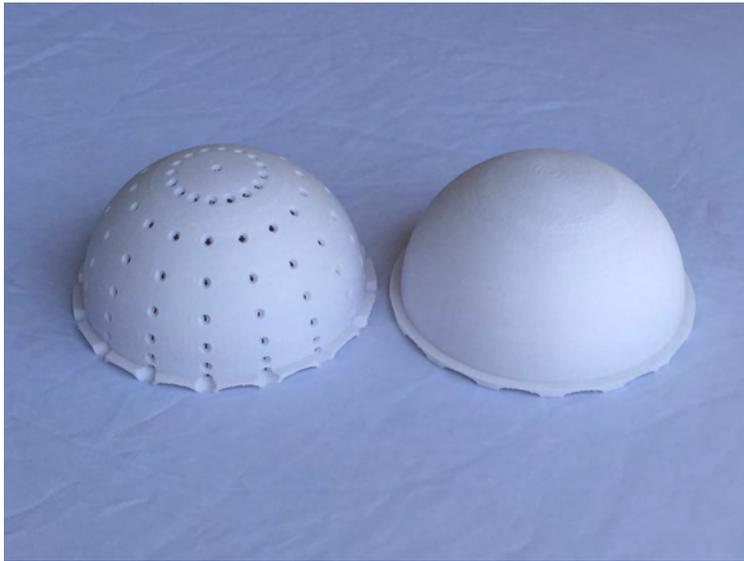
Figure 7.3: Example of using two separate prints for calibration. The dome on the left contains small holes designed to fit the LED perfectly for easy alignment.
