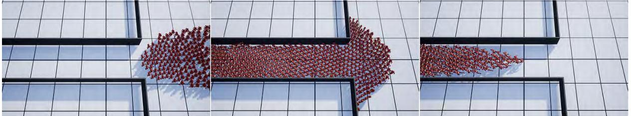
Figure 6.6: A group of agents passing through a narrow corridor. Left: Agents huddle on approaching corridor's entrance. Middle: A semi-circular arch forms as agents enter a narrow corridor. Right: Agents successfully exit.
