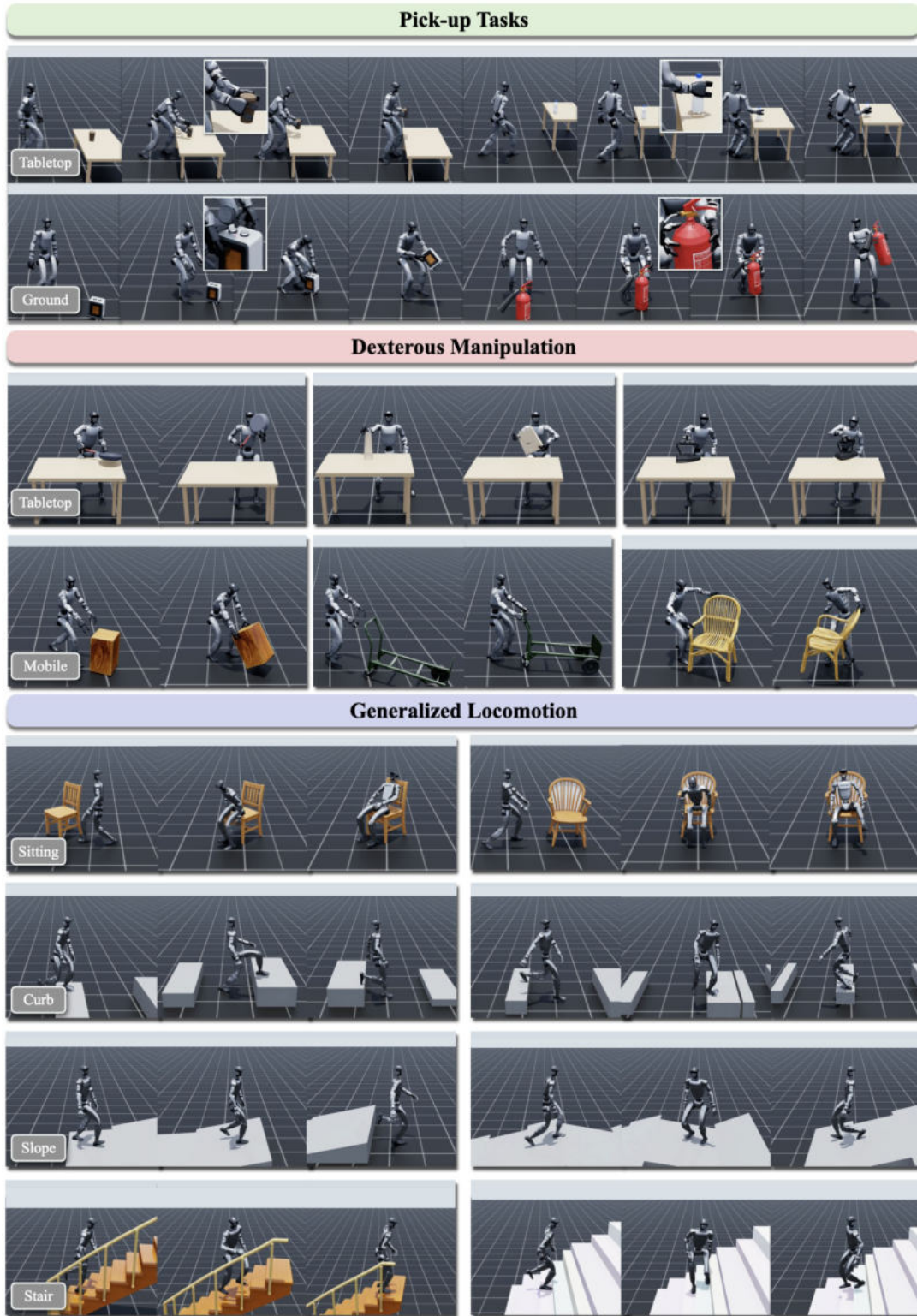
Figure 5.9: Diverse Loco-Manipulation Skills on the Unitree G1. We show representative results across pick-up (tabletop and ground), dexterous manipulation (tabletop and mobile), and generalized locomotion (sitting, curbs, slopes, and stairs).
