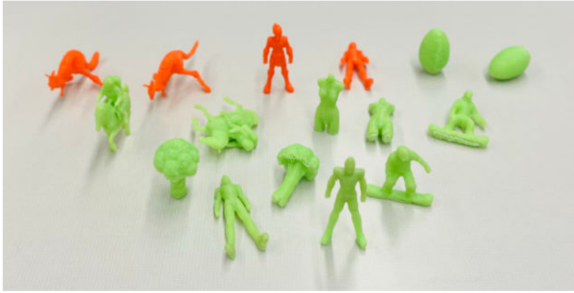
Figure 1.2: 3D-printed figurines created with Atlas3D stand stably, while those without Atlas3D have fallen down.
