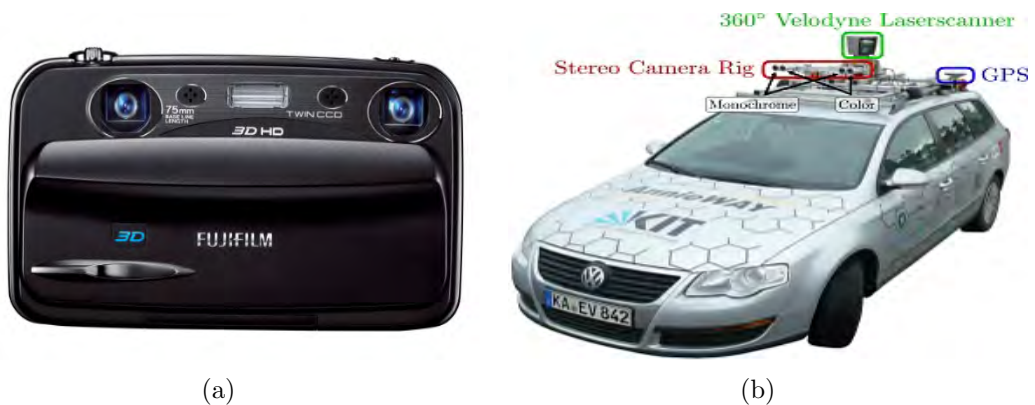
Figure 7.1: Fujifilm stereo camera and KITTI experimental vehicle.
