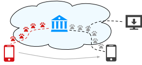
Fig. 3. Conceptual illustration of tracing-based solutions: consumer’s interests are forwarded toward the RV, they may meet the MP-trace along the way and move toward the MP without going through the RV.
