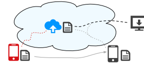
Fig. 4. Conceptual illustration of data depot: consumer interests are forwarded toward the depot to fetch data; they may meet the MP-trace on their way.
