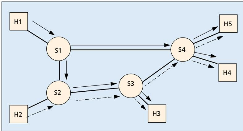
**FIGURE 1.** A simple network topology with the multicast routing trees. H1 and H2 are data sources, and H3, H4, and H5 are receivers. The solid lines depict the routing tree of H1; the dotted lines depict the routing tree of H2. In general, the set of sources and the set of receivers may overlap partially or completely. For the sake of clarity, here they are disjoint.
