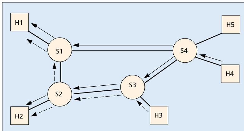
**FIGURE 2.** A simple network topology with the sink trees. *H1 and H2 are data sources, and H3, H4, and H5 are receivers (sinks). The dotted lines depict the sink tree of H3; the solid lines depict the sink tree of H4. For clarity the sink tree of H5 is omitted.*
