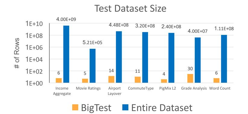
BigTest reduces tests by 10<sup>5</sup>X to 10<sup>8</sup>X, achieving 194X testing speed up.
