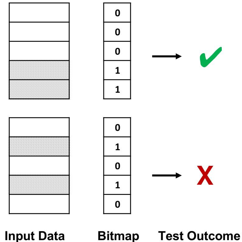
We use a bitmap based test memoization technique to avoid redundant testing of the same input dataset.
