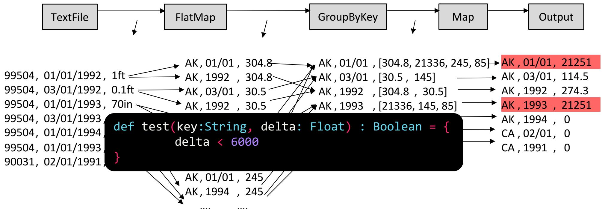
Given a test function, the goal is to identify a minimum subset of the input that is able to reproduce the same test failure.
