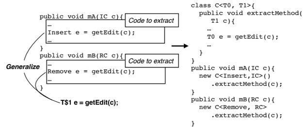
Fig. 5. Parameterize type refactoring
