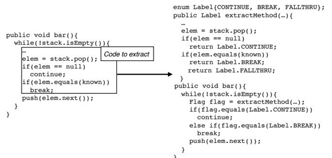
Fig. 8. Introduce exit label refactoring
