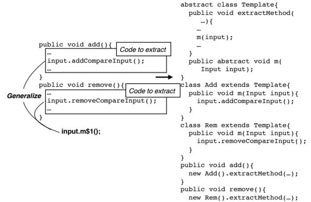
Fig. 6. Form template method refactoring
