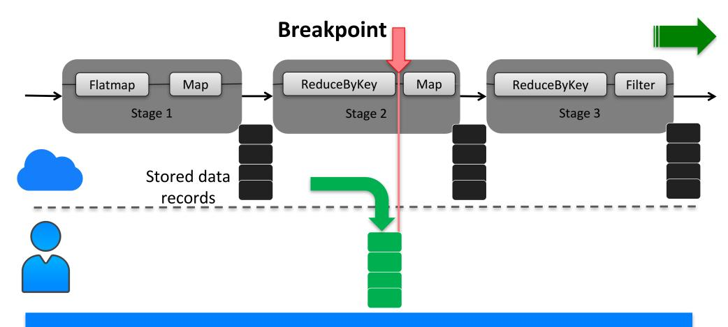
Simulated breakpoint replays computation from the latest materialization point where data is stored in memory
