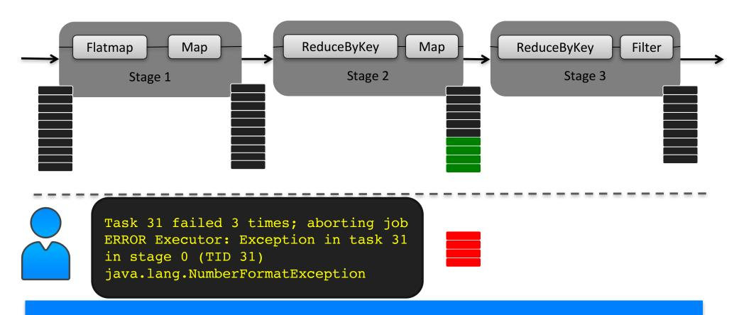
A user can either correct the crashed record, skip the crash culprit, or supply a code fix to repair the crash culprit.
