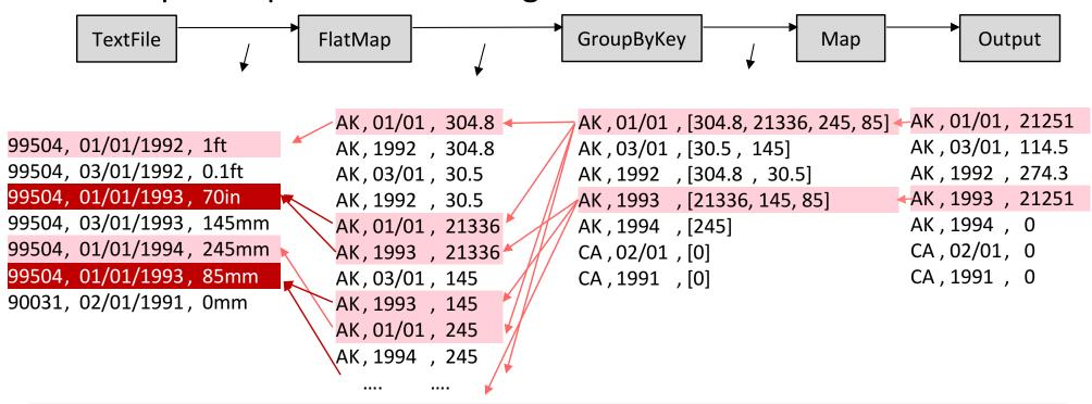
In case of multiple faulty outputs, BigSift overlaps two backward traces to minimize the scope of fault-inducing input records
