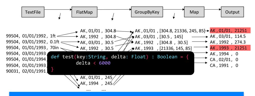
Given a test function, the goal is to identify a minimum subset of the input that is able to reproduce the same test failure.
