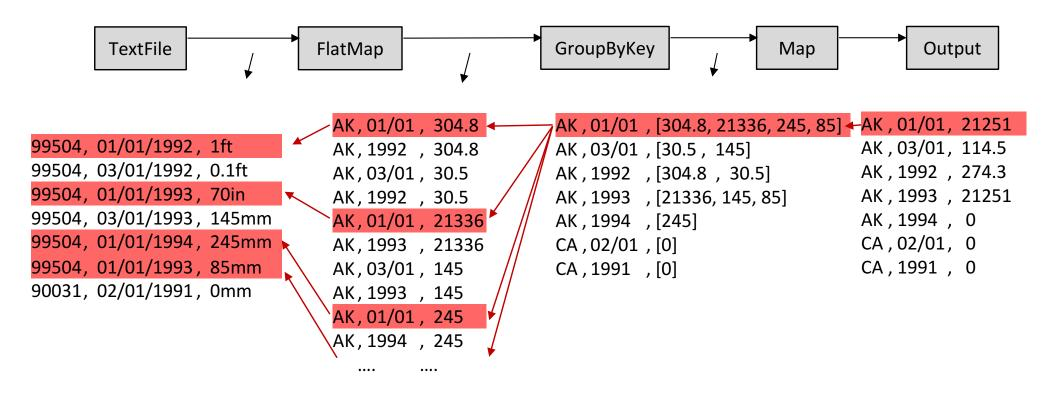
It over-approximates the scope of failure-inducing inputs *i.e.* records in the faulty key-group are all marked as faulty
