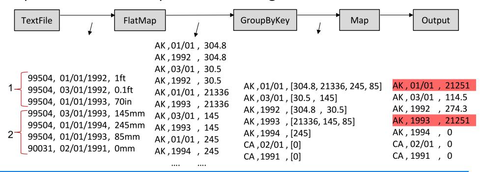
Delta Debugging performs a systematic binary search-like procedure on the input dataset using a test oracle function
