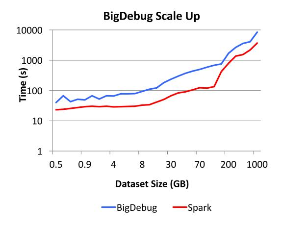
BigDebug retains scale up property of Spark. This property is critical for Big Data processing frameworks
