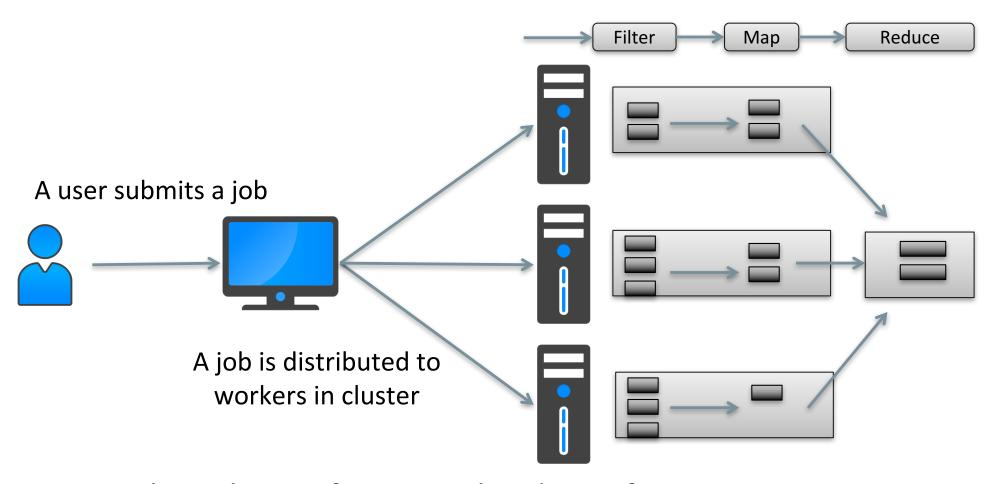
Each worker performs pipelined transformations on a partition with millions of records
