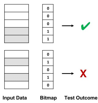
We use a bitmap based test memoization technique to avoid redundant testing of the same input dataset.
