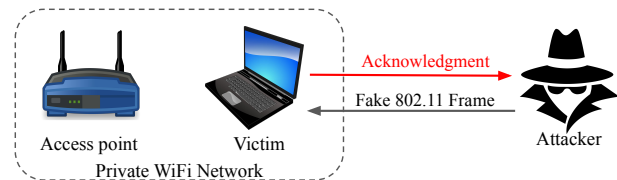
Figure 1: WiFi devices send an ACK for any frame they receive without checking if the frame is valid.
