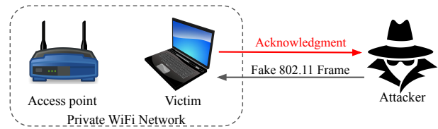
Figure 1: WiFi devices send an ACK for any frame they receive without checking if the frame is valid.
