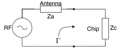
Figure 3: An equivalent circuit of an RFID tag.
