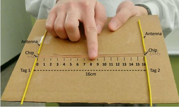
**Figure 6: Prototype device for sensing finger input: two RFID chips with dipole antennas are mounted 16 cm apart on a cardboard substrate, the chips are connected by copper tape to form a transmission line.**
