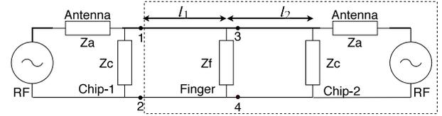
**Figure 8: An equivalent circuit of our input device.**
