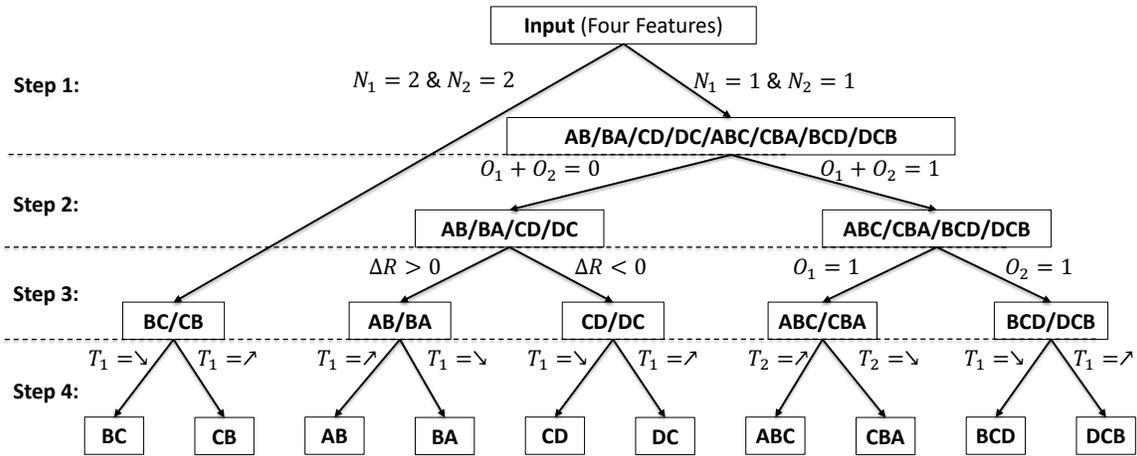
Figure 13: Sliding finger gesture detection algorithm decision tree.
