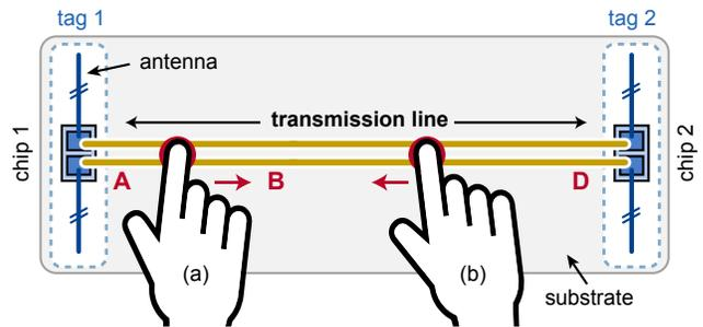
**Figure 1: The touch input sensing device is created by connecting the chips of two RFID tags together with copper strips to form a transmission line. When a finger is sliding in different directions between key known positions, e.g. (a) A-to-B or (b) D-to-B, relative RSS patterns for each chip can be used for gesture detection independent of changes to device location or RF environment.**
