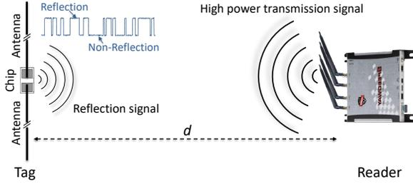
Figure 2: Illustration of a passive RFID system.
