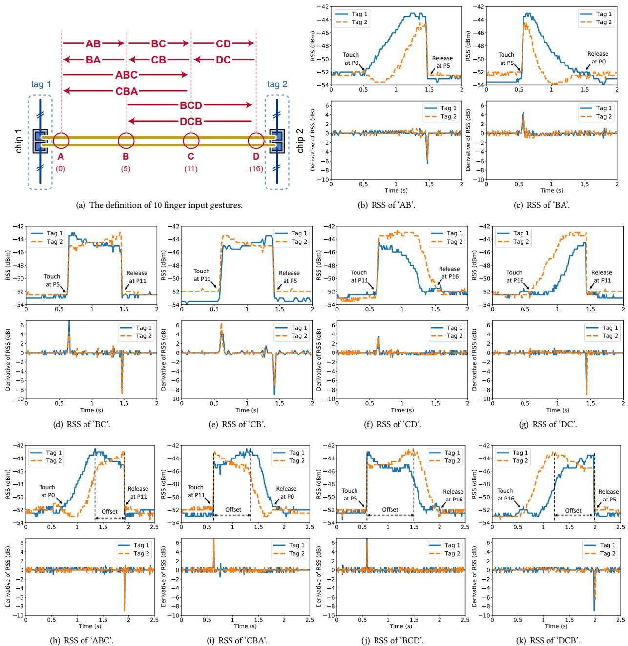
**Figure 11: Example sequences of RSS values and numerical derivatives resulting from the ten sliding finger gesture inputs.**
