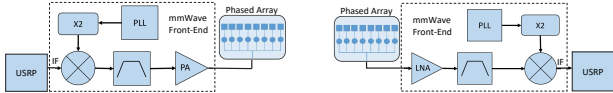
Figure 6: Agile-Link's Architecture. The figure shows block diagrams for both Agile-Link's transmitter and receiver.
