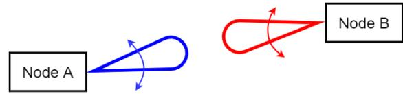
**Figure 1: mmWave devices need to focus their energy into beams, and align them to establish a communication link.**
