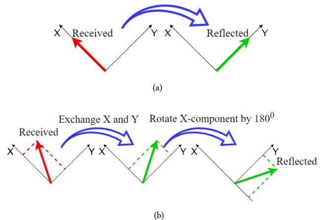
**Figure 6: Polarization Conversion. (a) if the polarization of the received signal is in X direction, mmTag’s node change it to Y direction and reflect it. (b) if the polarization of the received signal has an arbitrary direction, mmTag’s node change it to the orthogonal direction by exchanging the signal of X and Y port and performing a 180 degree phase shift on X.**
