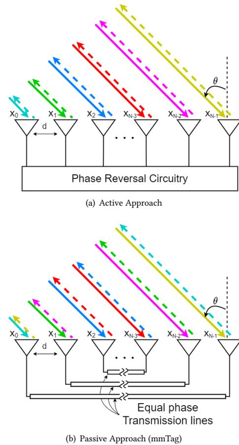
**Figure 3: Directional reflectors using two different approaches. The solid arrows show the received signal and the dashed arrows show the reflected signal of each antenna element. In (a) each antenna reflects its own received signal, while in (b) each antenna reflects the signal received by its mirrored antenna.**
