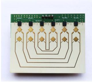
Figure 8: Our mmTag's node fabricated on PCB. The dimension of the node is only  $6 \times 5 \text{ cm}^2$  (i.e. smaller than a credit card).
