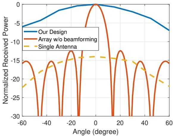
**Figure 11: mmTag’s Passive beamforming performance.** mmTag’s node reflects the signal back to the direction of the AP while experiencing minor loss across different angles respect to the AP. The figure also shows that the loss would be much higher if a fixed-beam array or a single antenna was used instead of mmTag’s design.
