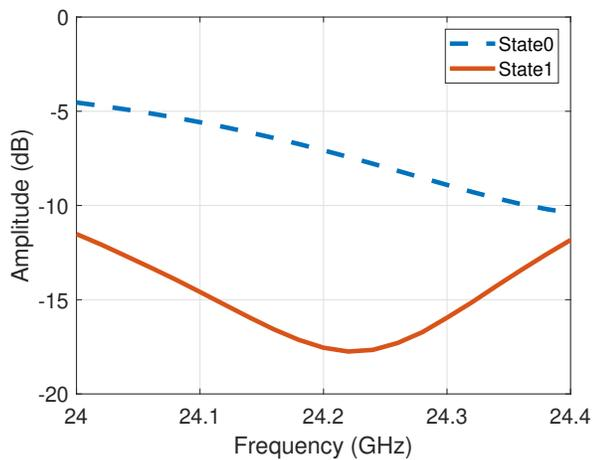
Figure 9: S11 coefficient of a node's antenna element for both states of the switch. In one state, antenna has low S11 at the carrier frequency of 24 GHz and hence it receives and reflects. In the other state, the antenna's S11 is high and hence it does not receive nor reflect.
