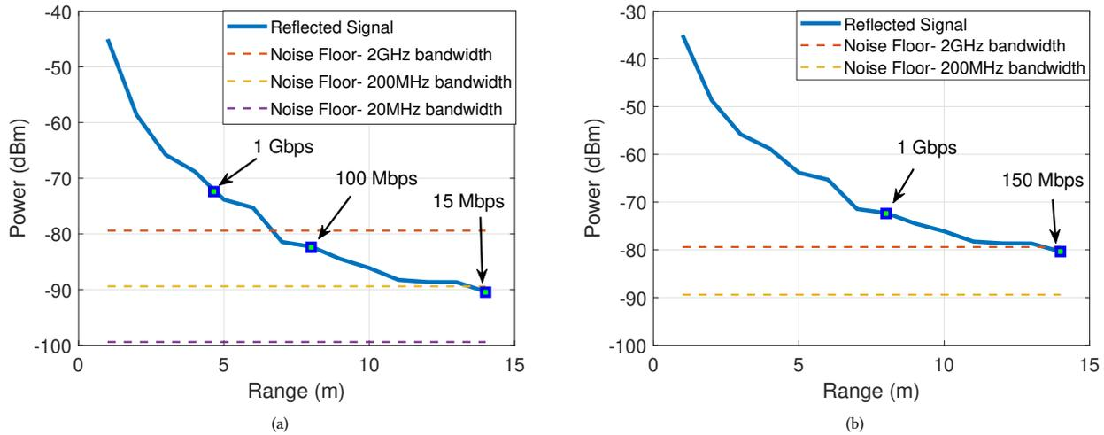
**Figure 13: mmTag range performance.** The figure shows the power of tag’s signal measured at the AP versus distance between the node and the AP for (a) AP is continuously transmitting the query signal and (b) AP is performing 10% duty cycling. The figure also shows the noise floor for different AP bandwidth as well as corresponding data rates for some signal powers.
