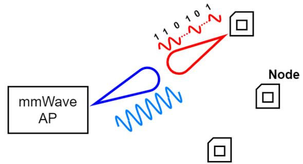
**Figure 2: mmTag AP scans the space by steering its beam. When the AP's beam is toward a node, the node modulates and reflects the AP's signal back in the direction of arrival.**
