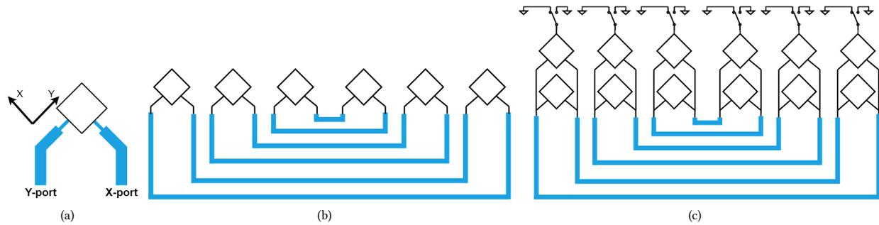
**Figure 5: mmTag’s node design. (a) our single element patch antenna with two port which enables operating in two different polarization. (b) our feed network design which enables the node to change the polarization of the received signal and then reflect it. (c) final design of mmTag where each antenna is connected to a switch to modulate the reflected signal.**
