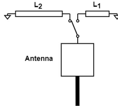
**Figure 4: Data Modulation.** mmTag's node uses a SPDT to switch between two transmission lines with different length. This allows the node to modulate the signal.
