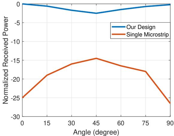
**Figure 12: mmTag’s polarization conversion performance.** mmTag’s node converts the polarization of a signal to its orthogonal polarization with minor loss for any orientation of the node. The figure also shows that the loss would be much higher if a typical patch antenna was used instead of mmTag’s design
