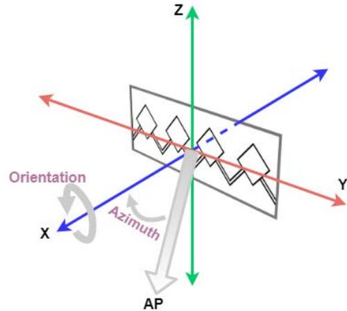
Figure 10: Evaluation Scenarios. We empirically evaluated mmTag for different ranges, orientations and angles of the node respect to the AP.
