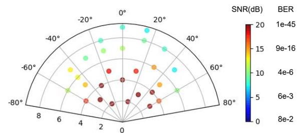
**Figure 14: mmTag System Performance.** mmTag enables high-SNR communication link between the AP and nodes for different scenarios (i.e. different range, orientation and angle of the node respect to the AP.)
