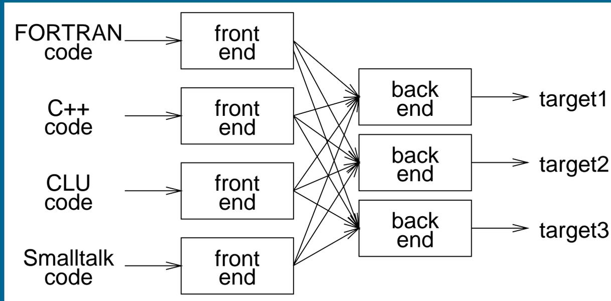
Can we build  $n \times m$  compilers with  $n + m$  components?
