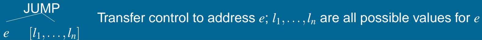
Transfer control to address  $e$ ;  $l_1, \dots, l_n$  are all possible values for  $e$
