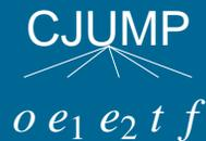
Evaluate  $e_1$  then  $e_2$ , yielding  $a$  and  $b$ , respectively; compare  $a$  with  $b$  using relational operator  $o$ :
