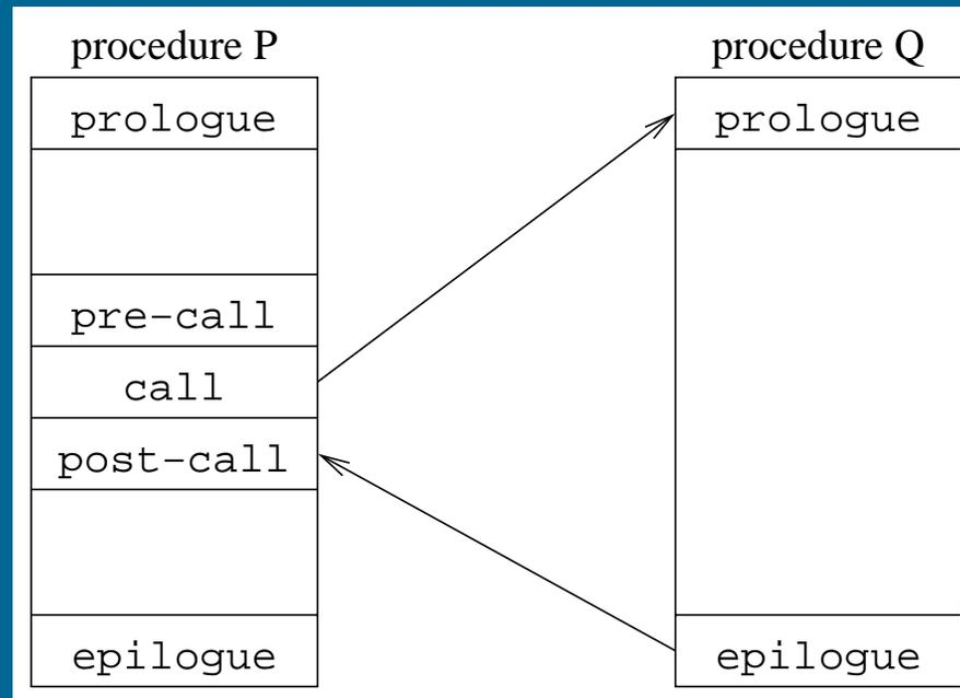
Each system has a *standard linkage*
