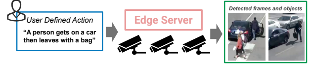
Figure 1: The high-level concept of a complex activity detection system: the user defines the rule then the system monitors incoming videos and outputs the matched frames.
