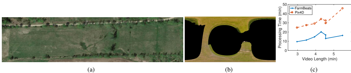
Figure 8: Orthomosaic Generation: (a) The Google Earth image for the farm in Figure 4. (b) Microsoft ICE image stitching pipeline fails to reconstruct it accurately. (c) Pix4D takes about 2.2x longer on average compared to our approach.
