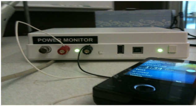
Figure 5: The hardware power meter used for energy measurements.
