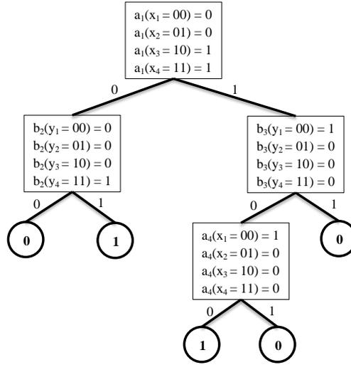
FIGURE 2.2: A protocol tree, where leaf nodes are represented by circles. At each internal node of the protocol, the function determines which branch of the tree to take (0 = left, 1 = right). The communication cost of the protocol is given by the height of the tree.
