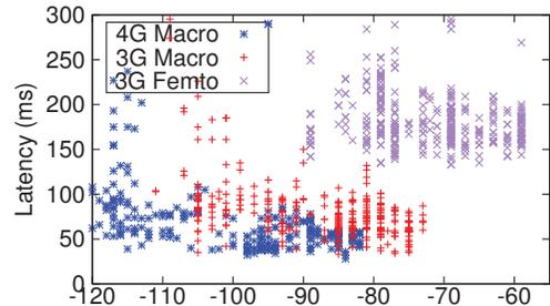
**Figure 5: Radio quality (RSSI/RSRP) versus ping latency collected by SpeedTest via 4G Macrocell, 3G Macrocells and 3G Femtocells. Note that Femtocells have relatively larger RSSI in vicinity.**
