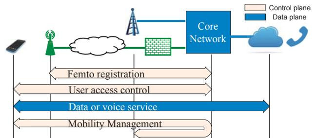
Figure 2: Main operations for Femtocells.
