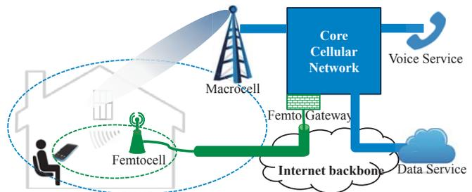
**Figure 1: Femtocells augment the Macrocell-based mobile network to boost coverage and capacity. Example: the user deploys a femtocell at home with poor Macrocell coverage.**
