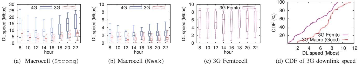
**Figure 4: Downlink data speed using 4G Macrocells, 3G Macrocells and 3G Femtocells in different scenarios. (a)(b)(c) show the boxplot of 5th, 25th, 50th, 75th, 95th percentiles at different hours of a day; (d) compares the CDF of downlink speed using 3G Femtocells and 3G Macrocells (8AM, 20-22PM) in Good coverage.**
