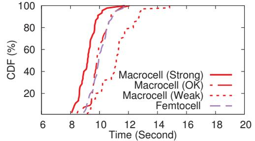
**Figure 6: Dial-to-ring delay using Femtocells and Macrocells at strong and weak zones.**
