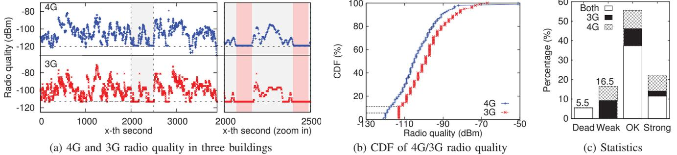
Figure 3: Macrocell radio quality in the indoor testbeds.
