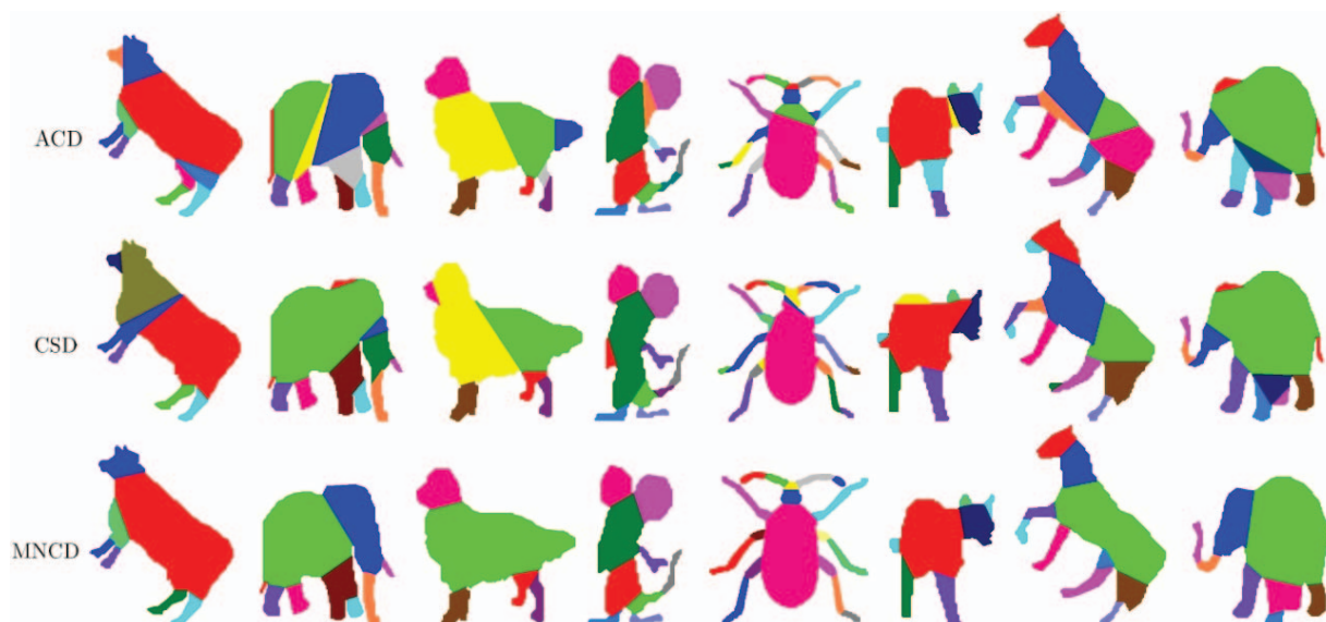
Fig. 8. Some decomposition results of ACD [7], CSD [8] and MNCD. Our MNCD method produces the least number of near-convex parts and our decompositions are visually more natural.
