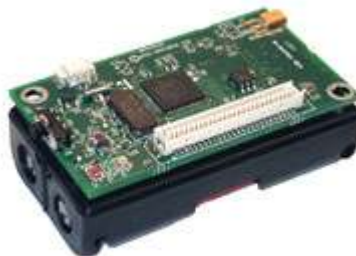
Figure 2. A Mica2 Mote without a sensor board attached.
