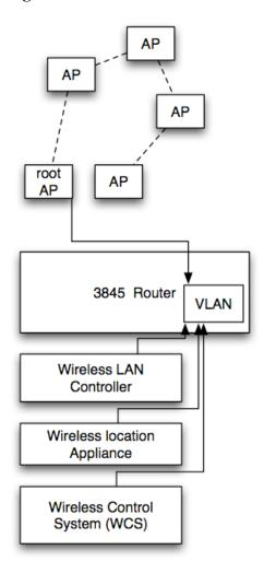
This diagram shows how the network components are connected. Mobile devices that connect to an AP generate packets with sensor data samples. The AP sends to packets through the root AP to the 3845 Router. The router then sends the packet to the Wireless LAN Controller, which processes the packets before sending them back to the router.
