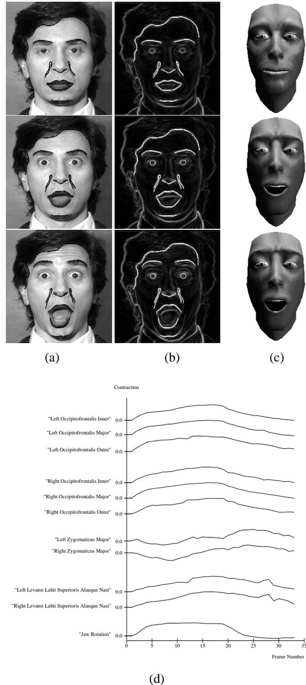
Figure 2: Dynamic facial image analysis and expression resynthesis. Sample video frames with superimposed deformable contours tracking facial features; (a) intensity images with black snakes, (b) image potentials with white snakes. (c) Facial model resynthesizes surprise expression from estimated muscle contractions. (d) Estimated facial muscle contractions plotted as time series.
