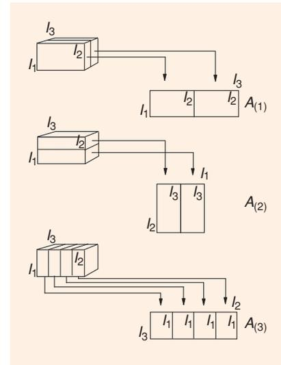
[FIG1] Flattening a third-order tensor. The tensor can be flattened in three ways to obtain matrices comprising its mode-1, mode-2, and mode-3 vectors.
