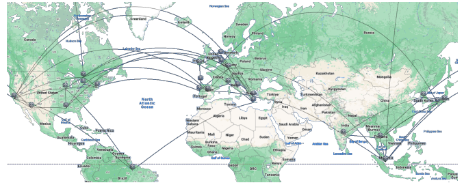
Fig. 6: The topology map of global NDN Testbed. Repo is deployed on every Testbed router.
