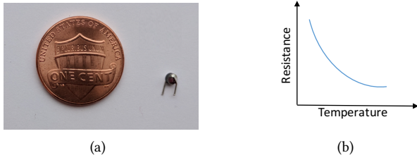
Figure 3: (a) An NTC thermistor used in our experiments, and (b) its functionality.
