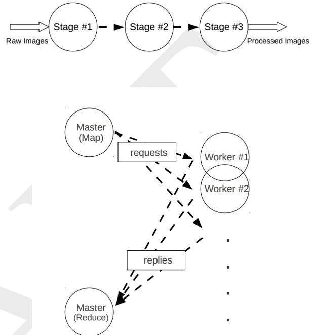
Figure 4. Patterns of actor programming (from top) (a) Pipeline pattern (b) Divide-and-Conquer pattern.
