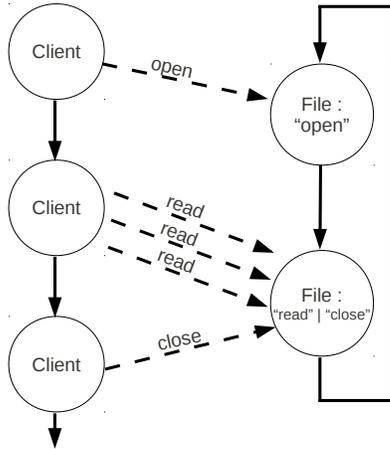
Figure 3. A file actor communication with a client is constrained using local synchronization constraints. The vertical arrows depict the timeline of the life of an actor and the slanted arrows denote messages. The labels inside a circle denote the messages that the file actor can accept in that particular state.
